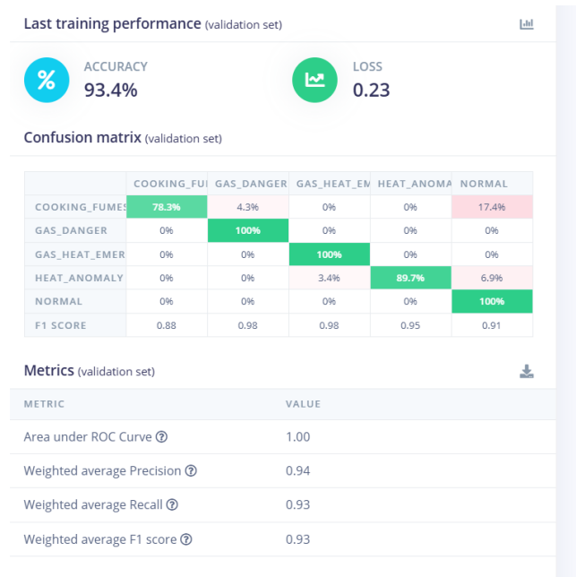
Figure 29: Training confusion matrix for the Edge Impulse classifier. The matrix shows strong classification performance for NORMAL, GAS_DANGER, and GAS_HEAT_EMERGENCY, with most ambiguity occurring around the intermediate COOKING_FUMES class.
